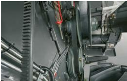
Threshing drum drive with two speed ranges which can be configured easily.
