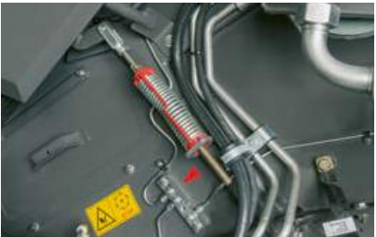
All lubrication points are combined and clearly indicated in grease anchor blocks.
