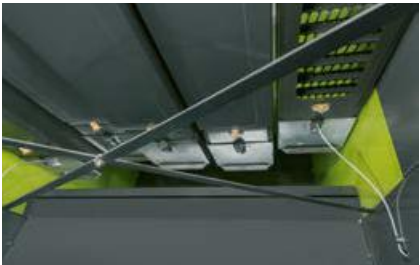
Maintenance openings at the end of the straw walkers provide fast access without tools.
