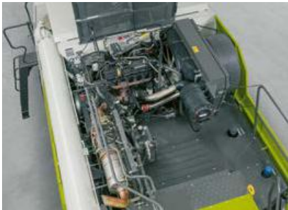
Cummins engine with AdBlue exhaust gas aftertreatment (Stage V)
