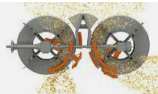
Power spreader for efficient straw spreading with minimal expenditure of energy.
