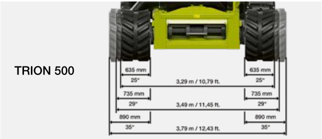
The 635 mm crawler tracks make the TRION compact on the road and so increase your mobility.
