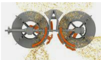
Power spreader for efficient straw spreading with minimal use of power.
