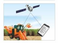
GPS enhancement provides SMS & web supervisor features which helps in finding the location of harvester and information on performance data.
